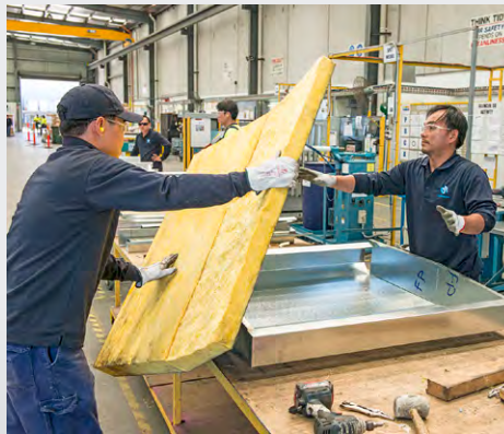
First layer of Bradford Ultratel installed in the baffle frame
