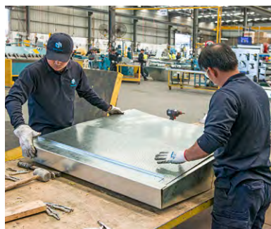
Acoustic baffle finished with perforated sheet metal
