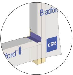
5. Once the tape is applied to the membrane on the building frame, remove the remainder of the liner from the other side and gently 'wipe' the tape onto the front face of the building frame.
