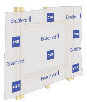
Establish the location of the window opening and cut diagonally from each corner at 45° toward the centre, joining the cuts with a short vertical cut in the centre of the panel, as required.
