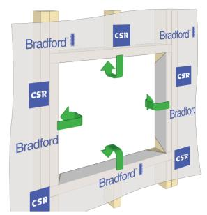
4. Pre-cut 100mm strips of Enviroseal ProctorWrap Flexi tape - partially remove the liner material when you are ready to commence application and apply the Flexi tape to the membrane on the building frame as illustrated.
