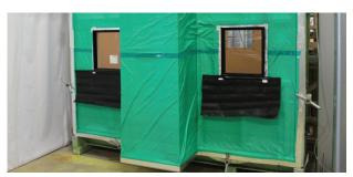
**82% reduction** in air infiltration was achieved when Thermoseal Wall Wrap was installed with overlaps, window frames, top plate and bottom plate sealed with tape.
