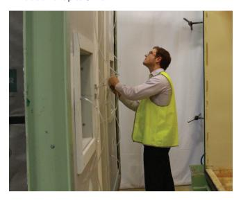
CSR Building Scientist Jesse Clarke, explained, "As part of our research into how wall wraps can improve the energy efficiency of a home, we designed an experiment to determine their impact on air infiltration through a typical residential wall".
