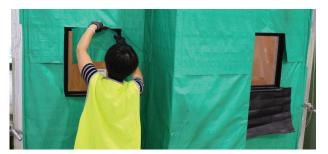
**20% reduction** in air infiltration was achieved when Thermoseal Wall Wrap was installed without any tape.
