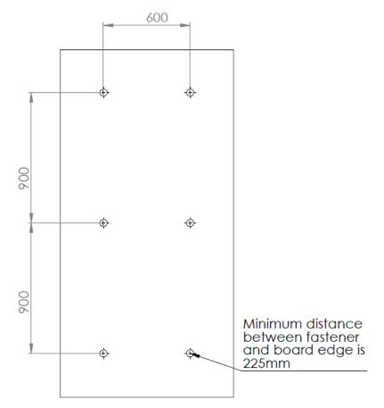
The board must be pinned in 6 places, spaced not larger than a 600mm x 900mm grid using Hilti X-IE Fasteners, or metal speed clips, or with screws and washers.
