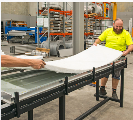
Martini Absorb is laid into the AcoustiSorb panel shell
