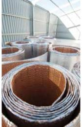
The special antiglare coating significantly reduces the heat gain inside a shed by reflecting up to 95% of radiant heat flow. Bradford Polyair Unicell incorporates a 4mm thick internal cell structure that provides an engineered air cavity within the product. This cell structure reduces heat transfer from the antiglare outer foil surface to the inner silver foil surface.
