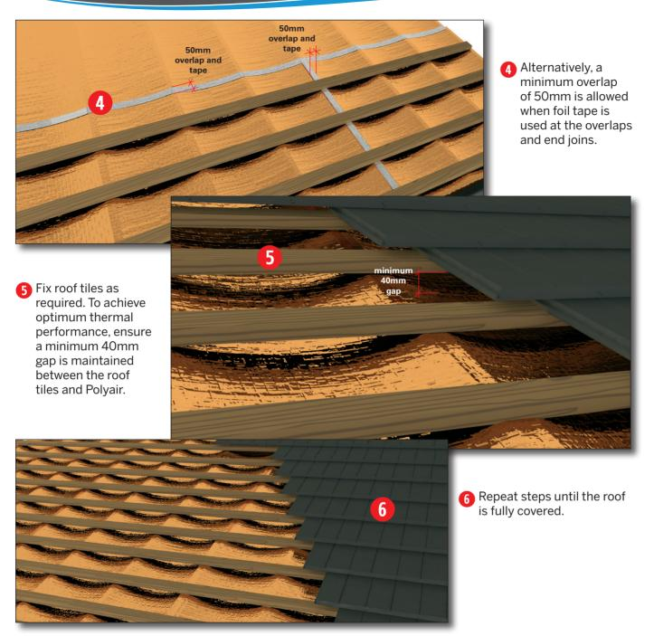
**Installation Guidance:** The install illustrations are a general guide only, for project specific advice contact the Bradford technical services team on 1300 850 305. Installation of Polyair should be in accordance with AS/NZS 4200.2 as a minimum. Refer to Polyair Technical Datasheets at reflectiveinsulation.com.au for handling, safety and product performance information.
