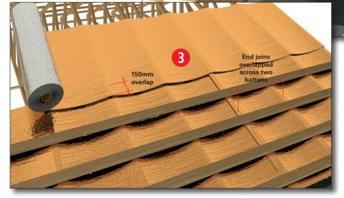
3 Overlap each row of Polyair by 150mm and ensure end joins are overlapped across two trusses or rafters. When reaching the top of the roof ensure Polyair is installed a minimum 150mm over the ridge line. See drawing 4 for taping options. Fix battens over the Polyair in sections as you go.
