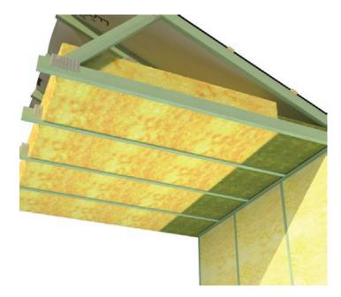
Stringing-in involves fixing straps onto the timber frame using a staple gun to ensure the ceiling batts are secured in place. Ensure that any staples that will be in contact with the plaster are fully embedded into the frame. Secure the strapping at 450mm intervals – except at the perimeter, where an additional strap will be required.
