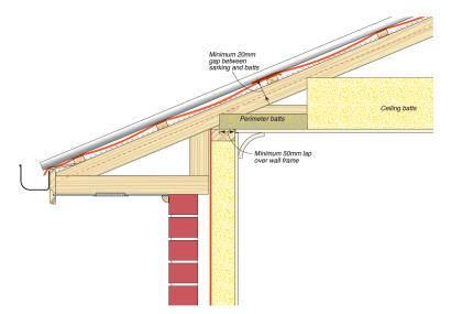
Maintain a minimum gap of 20 mm between the edge of insulation batt and the roof sarking or blanket/cladding to facilitate ventilation of roof space - do not compress the batts during installation.
