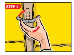
Swivel the Optimo aluminium strap 90° so the strap extends into the floor cavity between the joists and bend the strap upwards to support the insulation.
